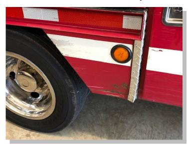
striping on the cab and body seems to have lost some of the reflectiveness and may not meet the NFPA1901 15.9.3.3.1 – "All retroreflective materials used to satisfy the requirements of 15.9.3.1 that are colors not listed in ASTM D4956, Section 6.1.1, shall have a minimum coefficient of retroreflection of 10 with observation angle of 0.2 degrees and entrance angle of -4 degrees."
