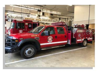
At first glance, the body looks faded and scratched from the rough terrain this vehicle has responded to. At closer examination, the rubber seals on for the compartment doors are dry rotted and are worn to a point of ineffectiveness. There is a moderate to major dent in front of the passenger side rear tire. The safety reflective
