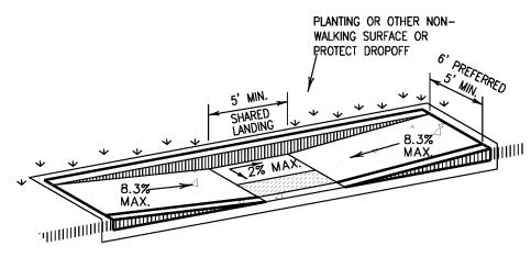
PARALLEL CURB RAMP (USE ONLY WHERE WATER WILL NOT POND IN THE LANDING.)  $T \times DOT \ TYPE \ 2$
