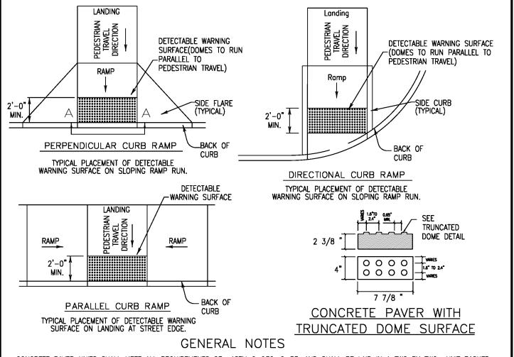
CONCRETE PAVER UNITS SHALL MEET ALL REQUIREMENTS OF ASTM C-936, C-33, AND SHALL BE LAID IN A TWO BY TWO UNIT BASKET WEAVE PATTERN, UNLESS SHOWN OTHERWISE IN THE PLANS.
