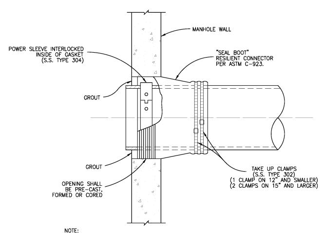
1. INSERT-A-TEE MAY BE USED IN LIEU OF SEAL BOOT FOR FIBERGLASS MANHOLES.
