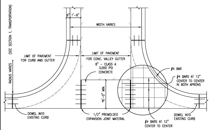
VALLEY GUTTER DETAIL FOR MID-BLOCK CROSSINGS, ARTERIAL STREETS, COLLECTORS, CROSSING PERPENDICULAR TO TRAFFIC FLOW
