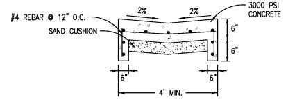
TYPICAL CONCRETE PILOT/TRICKLE CHANNEL
