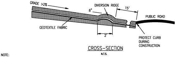
1. DESIGN AND MAINTENANCE SHALL BE ADEQUATE TO PREVENT SEDIMENT FROM ENTERING THE ROADWAY.
