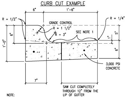
IF THE REMAINING CURB AND GUTTER SURFACE IS CHIPPED OR DAMAGED DURING REMOVAL AT THE NEW SAW CUT, THE ENTIRE GUTTER SECTION MUST BE REMOVED.
