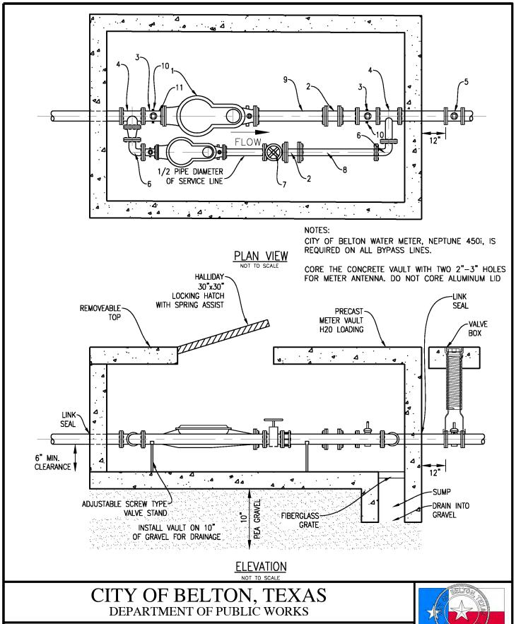
METER VAULT LAYOUT FOR 2" AND LARGER WITH AND WITHOUT BYPASS
