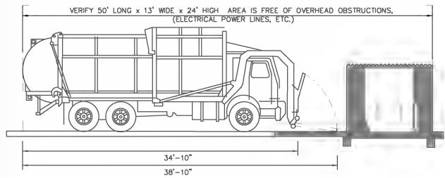
VEHICLE SHOWN IS A STANDARD 40 CY FRONT END LOADING COLLECTION TRUCK, ACTUAL DIMENSIONS WILL DIFFER BASED ON TRUCK MANUFACTURER, COORDINATE DESIGN WITH COLLECTION PROVIDER.
